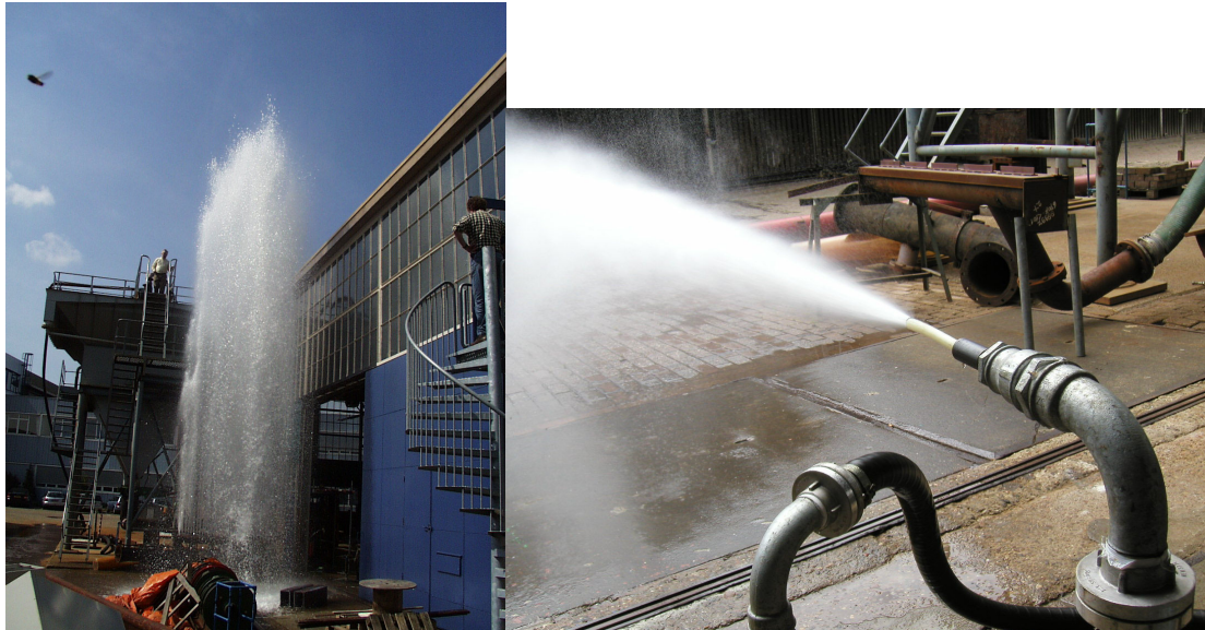
Fig. 6: Testing the jetwater distribution from the manifold and the sealing between tooth and adaptor.
